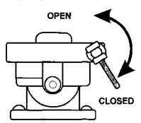
In order to move the mower from its storage area to a safe place to start it, you must open the pump bypass valves on each pump. Open each valve by turning it one turn counter clockwise. When you've moved the mower to its desired position, close each valve by turning it clockwise.
