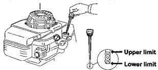
Running the engine with a low oil level will cause engine damage.
