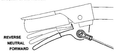
The mower will quickly respond to the position of the levers. To avoid abrupt changes of direction, squeeze the levers slowly rather than treating them like a switch. Operate the mower with the ground speed selector levers in their SLOW position until you are completely familiar with the sensitivity of the direction control levers.
