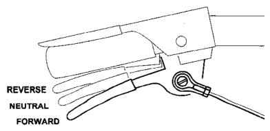
The direction control levers independently control each drive wheel for steering, slowing, and reversing. Squeezing the levers toward the hand grips slows the mower from the maximum forward speed. Squeezing the levers further to their neutral position stops forward motion. Squeezing the levers past neutral reverses direction.
