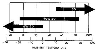
SAE 10W-30 is recommended for general, all-temperature use. Other viscosities shown in the chart may be used when the average temperature in your area is within the indicated range.
