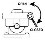
There is one very important thing to remember when transporting your mower: when you open the pump bypass valves to move the mower without the running engine, you disable all braking action. For this reason:
