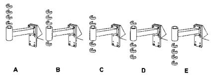
The front caster wheels are adjustable within their range in increments of 1/2 inch by changing the position of the four spacers on each caster post. The following table shows the position of the spacers for the various cutting heights.
