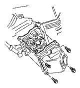
2. Install a 6x8 mm bolt in the threaded hole of each rocker shaft to hold the shaft in position. (The shaft can fall out when the piston is at firing position. One of the 6x26 mm valve cover bolts may be used to keep the shaft from falling out, but it will not keep the shaft in position.)
