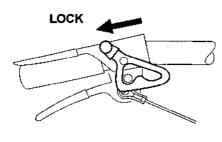
The neutral locks hold the direction control levers in their neutral position. Pulling the locks rearward prevents the direction control levers from going into their forward position. The levers can still be squeezed for reverse, however. When the neutral locks are engaged and you release the levers after reversing, they will return to neutral.
