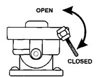
The bypass valves on each drive pump allow you to move the mower when the engine is not running. Open the valves by turning them one turn counterclockwise. See pages 16,24.
