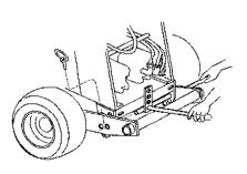
Install the linchpin(s) in the adjusting bar. Place the adjusting lever in its storage position and secure it with its spring pin.
