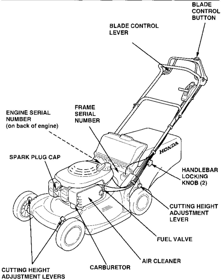
Record the frame and engine serial numbers in the space below. You will need these serial numbers when ordering parts and when making technical or warranty inquiries (see page 90).
