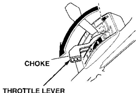
2. The choke arm should move counterclockwise, until it contacts the stop post on the carburetor.
