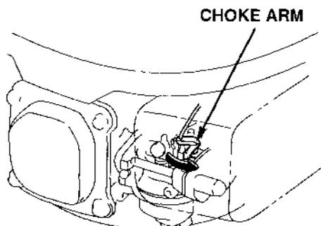
4. If the choke arm does not move all the way to its stop, in either direction, take the mower to an authorized Honda servicing dealer. Throttle cable adjustment involves related control plate adjustments.
