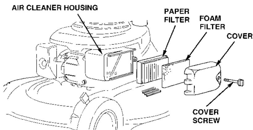
1. Unscrew and remove the air cleaner housing cover screw, then remove the air cleaner housing cover.
