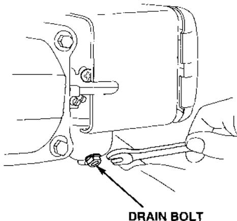
3. After the fuel is completely drained, reinstall the drain bolt.
