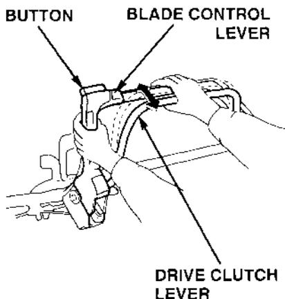
When moving and using the drive clutch lever to change self-propelled speed, continue to fully hold the blade control lever against the handlebar. This will help to extend the service life of the blade control mechanism.
