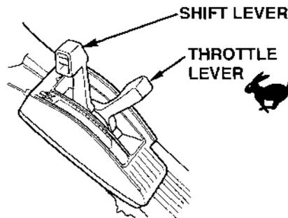
3. Start the engine and move the throttle lever to the FAST position.
