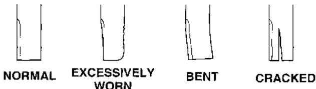
A dull blade can be sharpened, but a blade that is worn out, bent, cracked, or otherwise damaged must be replaced. A worn or damaged blade can break, causing blade pieces to be thrown from the mower.
