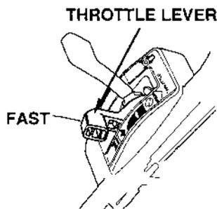
When you need to empty the grass bag or leave the mower for any reason, move the throttle lever to the STOP position.
