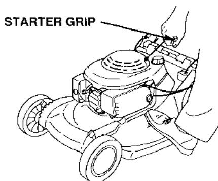
4. If the CHOKE position was used during starting, move the throttle lever away from the CHOKE position as soon as the engine warms up enough to run smoothly without use of the choke. Set the throttle lever at FAST to mow or at SLOW to idle.
