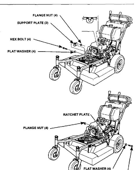
Remove the front bolt, washer and nut from the height adjustment ratchet plate.
