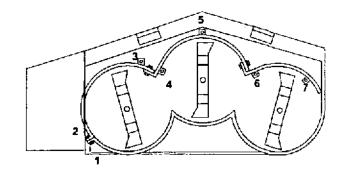
Install standard blades using the standard collars. Be sure to use the standard collars to maintain correct cutting height.
