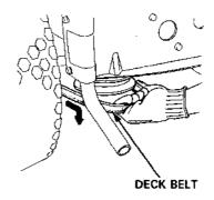
CAUTION: When the cutter deck is removed, the return spring will cause the deck height adjusting lever to snap unward when the release button is pressed. Hold the lever firmly, and carefully return it to the UPPER position after removing the deck.
