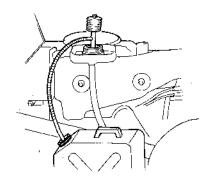
Turn the fuel valve ON, loosen the carburetor drain screw, and drain the fuel into an approved gasoline container. After draining tighten the drain screw securely.
