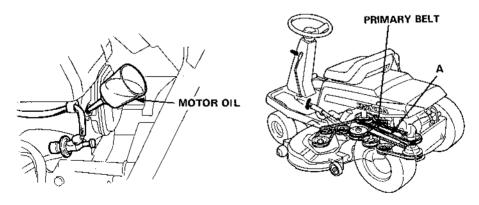
CAUTION: Be sure to wear heavy gloves when pulling the primary belt. If the riding mower has been running, the engine will be very hot. Allow it to cool before proceeding.
