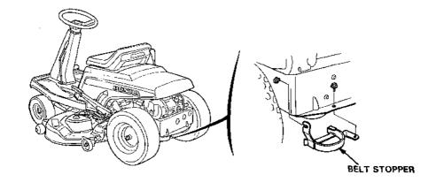
4-2. Remove the primary belt from the pulley on the underside of the transmission.
