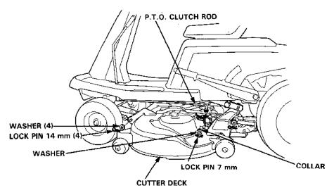
4-5. Remove the front deck arms from the frame body by removing the two lock pins and washers.
