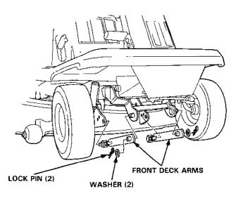
4-6. Disengage the cutter deck from the rear deck arms by moving it from side to side.
