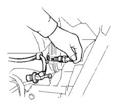
7. After a new spark plug has been seated by hand, it should be tightened 1/2 turn with a wrench to compress its washer.
