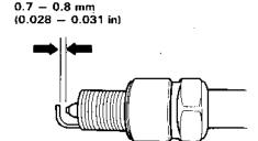
6. Thread the plug in by hand to prevent cross threading.
