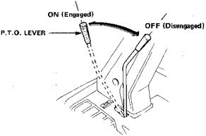
NOTE: An interlock switch prevents the engine from starting unless the P.T.O. lever is in the OFF position.
