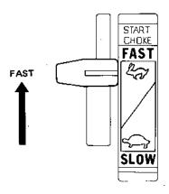
NOTE: The riding mower can be operated at intermediate throttle settings if desired, but always maintain sufficient engine speed for good pulling power and efficient blade operation. Use the shift lever to select the desired driving speed range.
