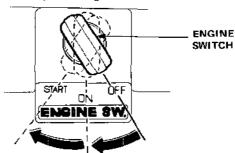
NOTE: The starter motor will not work unless the shift lever is in NEUTRAL and the P.T.O lever is in the OFF (Disengaged) position.
