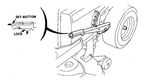
2. Move the throttle lever to the FAST position.
