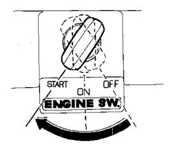
CAUTION: Do not use the starter motor for more than 5 seconds. If the engine fails to start, release the key, and wait at least 10 seconds before operating the starter motor again.
