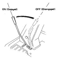
4. Move the shift lever to select the desired gear position. The clutch will engage automatically in about one second.
