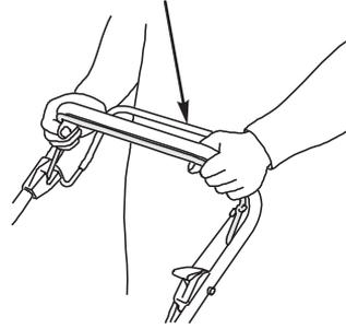
2. Pull back on the flywheel brake lever and hold it against the handlebar.
