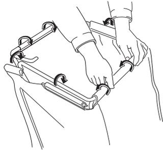
Lift the rear door, remove the mulching plug, then install the grass bag.
