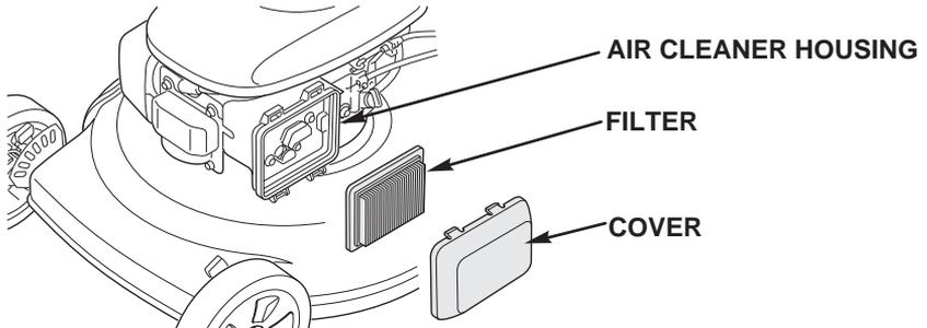
1. Press down on the cover tabs, then remove the cover. Remove the filter and inspect it; if damaged, replace the filter.
