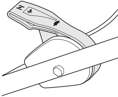
When you need to leave the mower for any reason, move the throttle to SLOW, then turn the engine OFF by releasing the flywheel brake lever.
