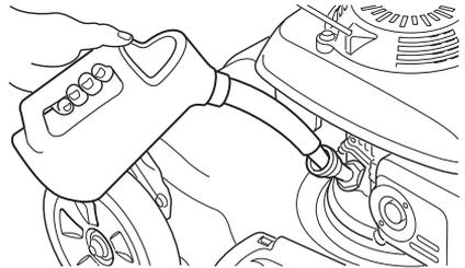
4. Fill with the recommended oil. Do not overfill; measure the oil level as shown on page 34.
