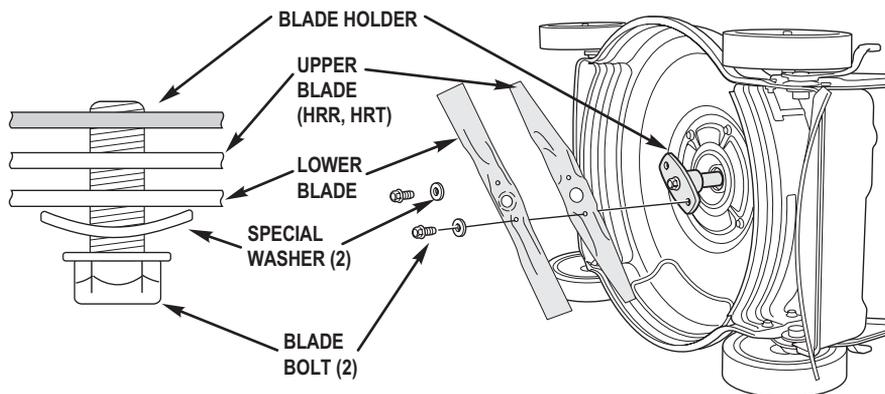
3. **Installation:** Clean around the blade holder. Install the blade(s) using the bolts and special washers as shown (concave side of the special washers toward the blade(s)).
