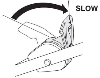
Release the drive clutch lever (SD, S3D).
