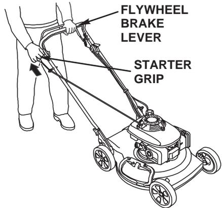
Keep your hands and feet away from the mower deck at all times when starting and running the engine.
