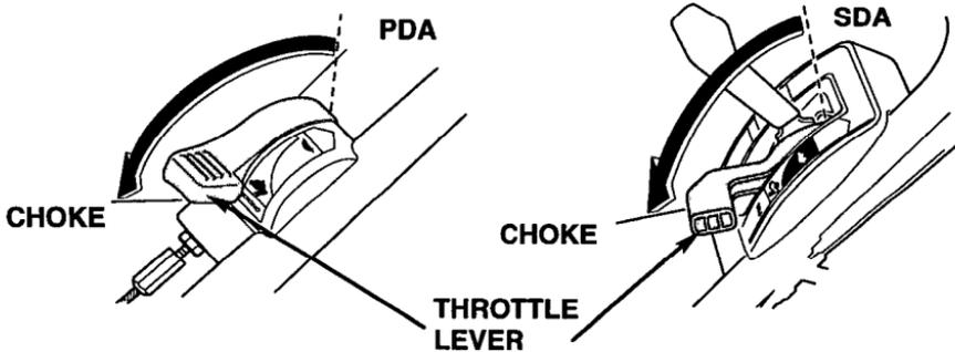
2. The choke arm should move counterclockwise, until it contacts the stop post on the carburetor.
