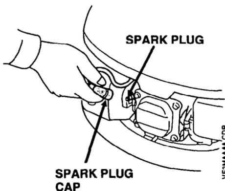
2. Remove the spark plug with a 21 mm ( $13/16$  in) spark plug wrench.
