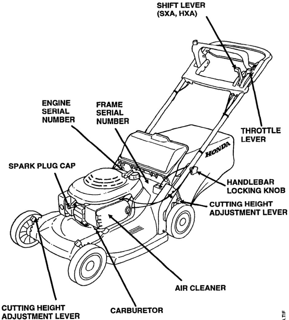
Record the frame and engine serial numbers in the space below. You will need these serial numbers when ordering parts and when making technical or warranty inquiries (see page 81).
