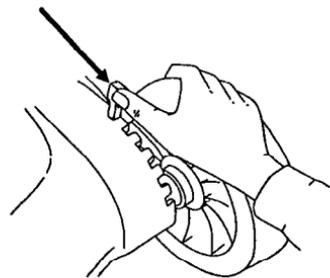
If you are not sure what cutting height to select, start with a high setting and check the appearance of the lawn after mowing a small area. Then readjust cutting height if necessary.
