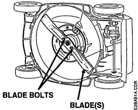
Inspect the blade(s) for wear and damage.
