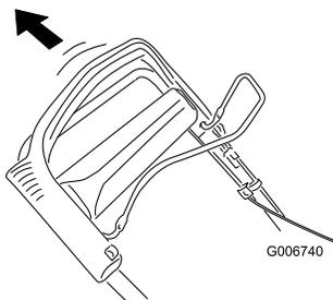
3. Pull the cable jacket downward until you remove the slack in the exposed cable (Figure 28).
