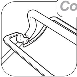
Operate all control levers several times and ensure that the cables move freely. Check that the engine stop and (ground drive clutch levers - **Autodrive models**) return freely to their rest position when released.
