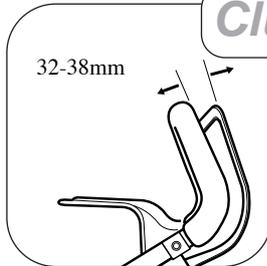
**Autodrive Models** - Check the clutch cable operation every 25 operating hours and adjust if necessary. The clutch cable is adjusted correctly when the belt drive just engages with the clutch lever positioned 32-38mm from the handlebar.
