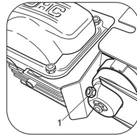
Disconnect the spark plug lead.
