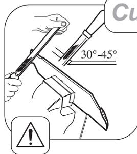
A slightly worn cutterblade may be re-sharpened. Both blade edges must be sharpened equally to ensure balance. Sharpen the cutterblade every 25 mowing hours or more frequently if conditions require. Remove the cutterblade from the mower and clean using a brush and water. Inspect the cutterblade for signs of damage. Sharpen both cutting edges with a flat file to restore performance.
