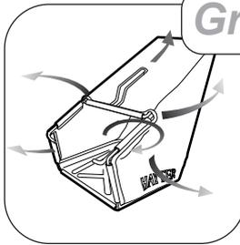
Lift the grassbag through the handlebar and close the rear deflector to rest against the rear of the mower. To empty the grassbag, pour out the grass clippings and shake the grassbag vigorously to clean the airways. Good grass collection depends on good air flow through the grassbag. When collecting grass clippings it is important that the grassbag is emptied regularly to prevent blockages and engine overloading.
