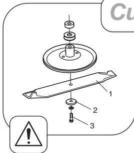
Assemble the cutterblade (1) with the turned up edges facing towards the engine. Secure the cutterblade using the friction washer (2) and new fixing bolt (3) and tighten to a torque of 54Nm.
