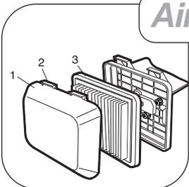
To service the air cleaner remove the air cleaner cover (1) by releasing two top catches (2) and tilting away from body until lower tabs release. Remove cartridge (3) and clean by tapping gently on a flat surface. If very dirty or damaged replace.
