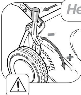
To prevent engine overloading and blockages be prepared to make two cuts in areas of heavy growth. If collection is required, first mow the area at the maximum height of cut setting with the grassbag fitted. Reduce the height of cut and mow the area again as necessary until the required finish is obtained.
