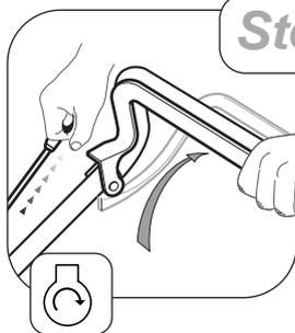
Stand behind the mower and hold the handlebar with your left hand together with the engine stop lever. With your right hand hold the engine start - grip and pull slowly until resistance is felt, then pull rapidly to crank the engine. Carefully return the start grip to the storage position when the engine starts.
