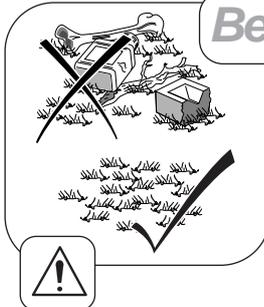
To prevent accidents thoroughly inspect the area and remove all objects which when contacted by the cutterblade could become dangerous projectiles. Inspect the area for hidden obstructions which when contacted by the cutterblade could risk health and safety or result in damage to the mower. Remember the location of these obstructions and ensure that you mow around them.
