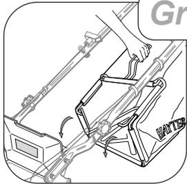
Raise the rear deflector, lower the grassbag through the handlebar and hook in position. Lower the deflector to rest on the grassbag.
