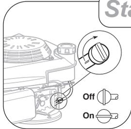
Turn the fuel valve to the on position. Move the throttle control lever to the 'choke' position before starting a cold engine. Move the throttle control lever to the 'fast' position before starting a warm engine.
