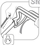
Stand behind the mower and hold the handlebar together with the engine stop lever with your left hand. With your right hand hold the engine start - grip and pull slowly until resistance is felt, then pull rapidly to crank the engine. Carefully return the start grip to the storage position when the engine starts.
