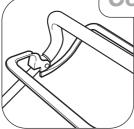
Operate all control levers several times and ensure that the cables move freely. Check that the engine stop and ground drive clutch levers return freely to their rest position when released.
