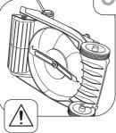
Drain the fuel by running the engine until the fuel tank is empty and the engine stops. **Remove the spark plug lead** and allow the engine to cool. Turn the mower on its left hand side and ensure that the air cleaner side of the engine is uppermost.
