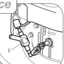
Check the spark plug gap with a feeler gauge and set at 0.50mm.
