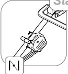
Move the throttle control lever to the 'choke' N position before starting a cold engine. Move the throttle control lever to the 'fast' position before starting a warm engine.
