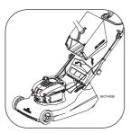
Raise the rear deflector, lower the grassbag between the handlebar and hook in position. Lower the deflector to rest on the grassbag.
