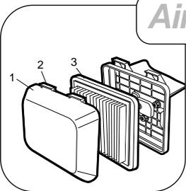
To service the air cleaner remove the air cleaner cover (1) by releasing two top catches (2) and tilting away from body until lower tabs release. Remove cartridge (3) and clean by tapping gently on a flat surface. If very dirty or damaged replace.
