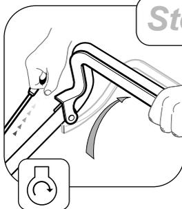
Stand behind the mower and hold the handlebar with your left hand together with the engine stop lever. With your right hand hold the engine start - grip and pull slowly until resistance is felt, then pull rapidly to crank the engine. Carefully return the start grip to the storage position when the engine starts.
