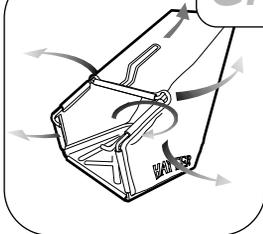
Lift the grassbag through the handlebar and close the rear deflector to rest against the rear of the mower.
