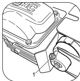
Disconnect the spark plug lead.
