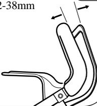
**Autodrive Models** - Check the clutch cable operation every 25 operating hours and adjust if necessary. The clutch cable is adjusted correctly when the belt drive just engages with the clutch lever positioned 32-38mm from the handlebar.
