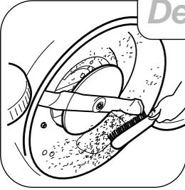
Remove grass debris from the top and underside of the deck housing immediately after use.
