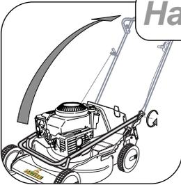
Unscrew the handlebar securing knobs sufficiently to allow the handlebar to pivot. Unfold the handlebar to the operating position. Tighten both handlebar knobs to secure the handlebar in position.
