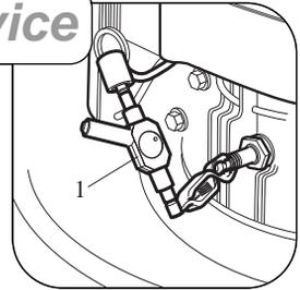
Check the spark plug gap with a feeler gauge and set at 0.76mm.
