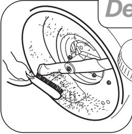
Remove grass debris from the top and underside of the deck housing immediately after use.
