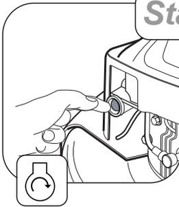
Push the primer button 5 times allowing 2 seconds between each push.
