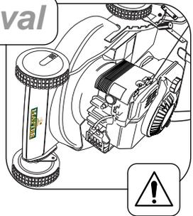
The condition of the cutterblade and its mounting arrangement should be checked regularly for signs of wear or damage. Ensure that the cutterblade is not bent or cracked.
