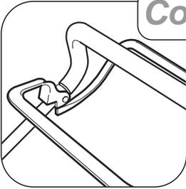
Operate all control levers several times and ensure that the cables move freely. Check that the engine stop and (ground drive clutch levers - **Autodrive model**) return freely to their rest position when released.
