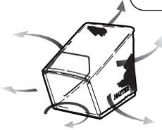
Lift the grassbag through the handlebar and close the rear deflector to rest against the rear of the mower.
