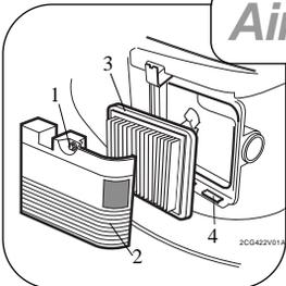
To service the air cleaner, loosen screw (1) and remove cover (2).
