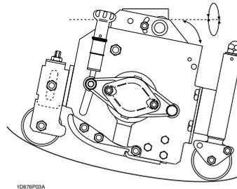
**Grass deflectors:** The rear grass deflectors must always be correctly fitted. The deflectors should be set as low as possible to deflect grass discharge to the ground.
