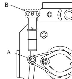
Tighten nut 'A' both ends.
