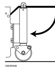
**Height of cut gauge:** An optional height of cut gauge is available to assist in achieving accurate cut height settings. It is suitable for both fixed and floating cutterheads.
