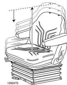
**Backrest adjustment:** Pull handle 'E' outwards to adjust the seat backrest angle. Release the handle to lock the seat backrest in position.
