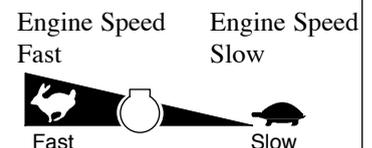
Note that the engine speed dictates the speed of the other functions, i.e. travel, cutting cylinder, position controls.
