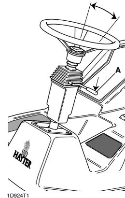
**Adjusting the length of the steering column:** Move the lever 'A' upwards to adjust the length of the steering column. Release the lever to lock the steering column in position.
