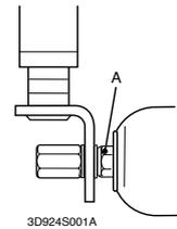
**Check cutterhead rear roller scraper wire tension:**
