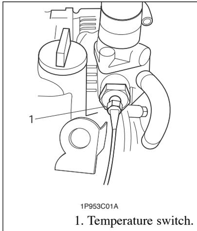
**Check the hydraulic oil overheat warning system:** Turn the ignition key to the 'ignition on' position 'I'. Disconnect the red/blue wire terminal from the hydraulic tank temperature switch and touch the metal terminal of the wire onto a suitable earth point, ensuring that the metal surfaces make good contact. The horn will sound and the hydraulic oil temperature warning light will illuminate to confirm correct operation. If the system is faulty, make repairs before operating the mower.
