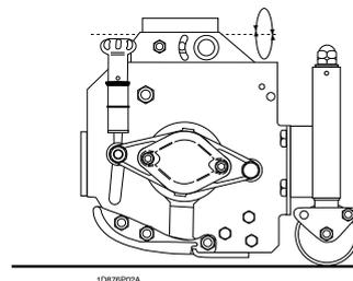
**Floating MK3 200mm Cutterheads:** When the mower is set up with floating cutterheads the height of cut is gauged by the front and rear rollers. The cutterhead is allowed to pivot fore and aft as well as laterally. This arrangement is recommended for high quality grass areas and performs well where grass is short and the ground undulations are severe.
