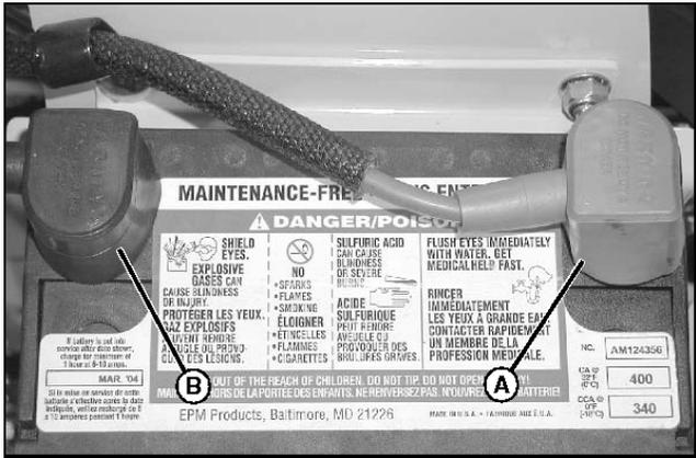
1. Connect positive (red) cable to battery positive (+) terminal. Install red terminal cover (A).
