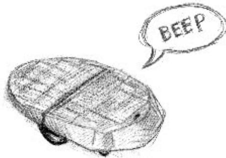
If the lawn mower avoids the shade during the day, it is because the batteries at the present time do not have sufficient capacity and to also ensure a long operating time. Large amounts of sun (sunny weather) allow the mower to charge fully before it starts to move, while small amounts of sun (cloudy) means that it charges a little and then moves hoping to find a sunnier part of the lawn.
