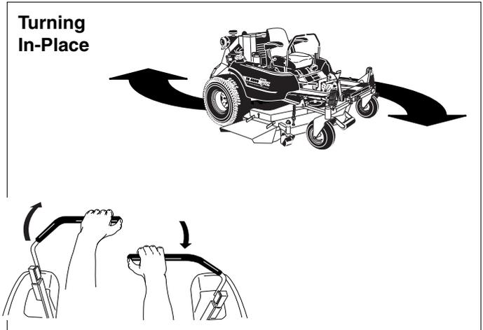
Figure 11. Turning in Place
