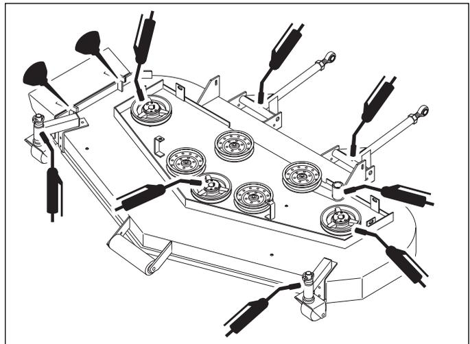
Figure 25. Deck Lubrication
