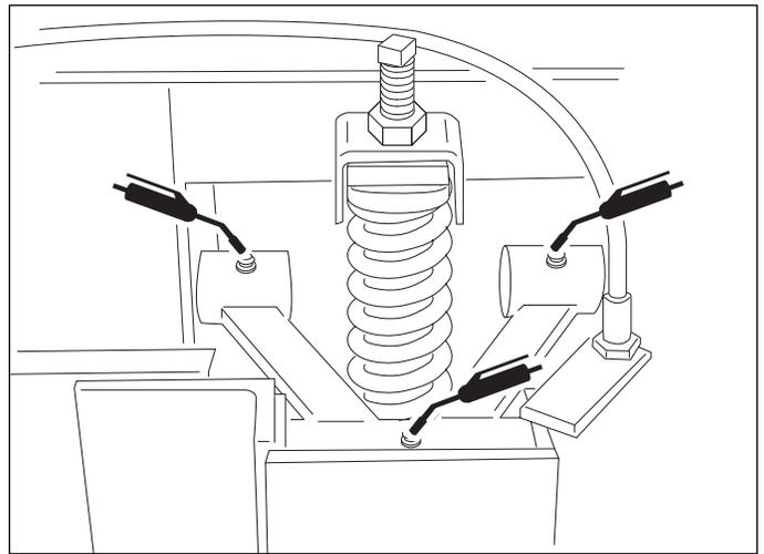
**Figure 29. Rear Suspension Lubrication**
