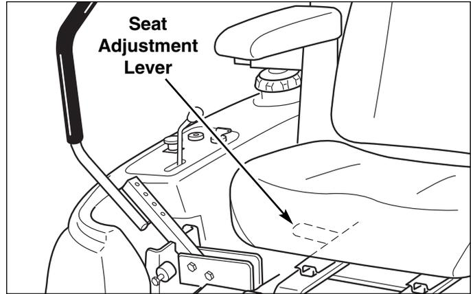
Figure 34. Seat Adjustment
