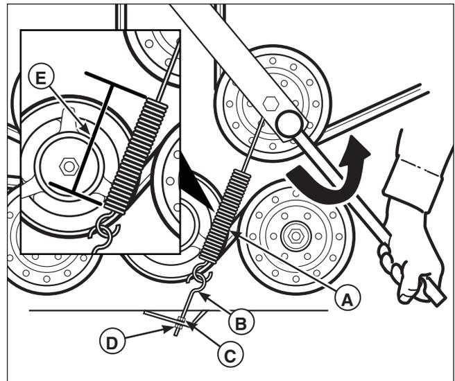
**Figure 51. Mower Belt Idler Spring Length**
