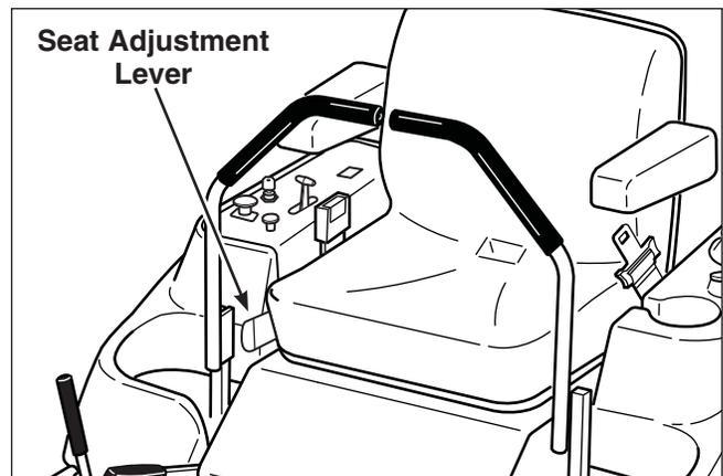
Figure 30. Seat Adjustment
