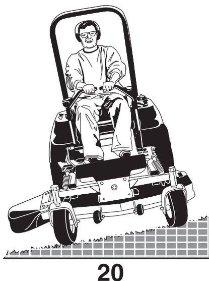
Operation on slopes can be dangerous. Using the unit on a slope that is too steep where you do not have adequate wheel traction (and control) can cause sliding, loss of steering, control, and possible rollover. You should not operate on a slope greater than a 5.4 foot rise over a 20 foot length (15 degrees).
