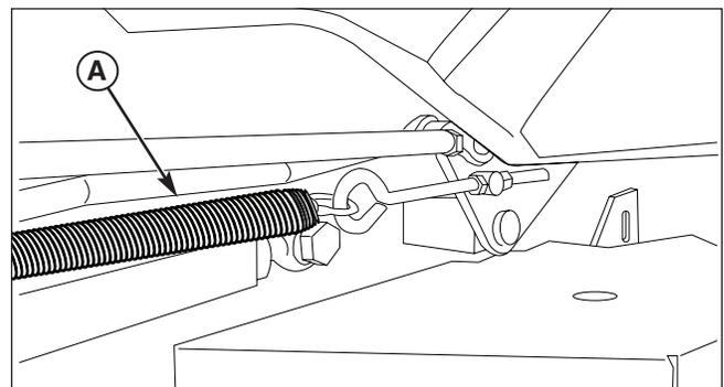
**Figure 42. Deck Lift Spring Location**
