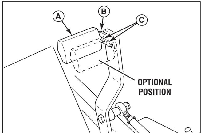
**Figure 36. Foot Pedal Adjustment**
