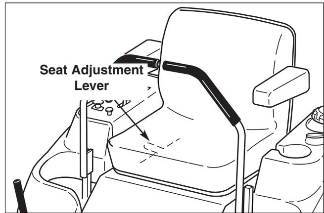
Figure 28. Seat Adjustment
