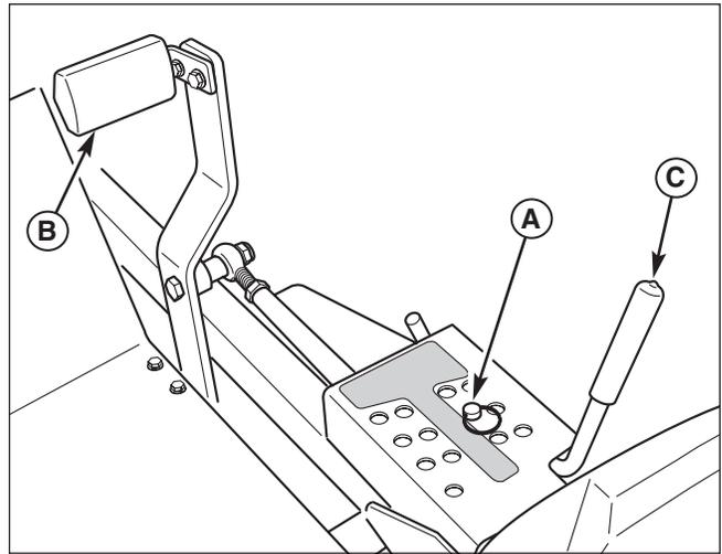
**Figure 35. Mowing Height Adjustment**
