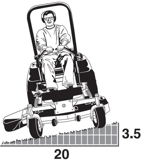
Operation on slopes can be dangerous. Using the unit on a slope that is too steep where you do not have adequate wheel traction (and control) can cause sliding, loss of steering, control, and possible rollover. You should not operate on a slope greater than a 3.5 foot rise over a 20 foot length (10 degrees).
