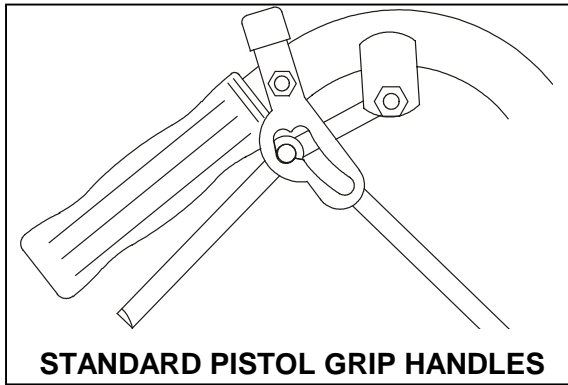
FIGURE 16 DRIVE LEVER AND LATCH IN NEUTRAL POSITION
