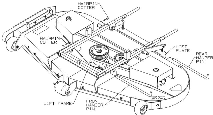
3. Slide deck from beneath chassis.
