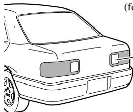
Check the position of your vehicle's reversing lamp (the one that lights up when the shift lever is in reverse [R]) and find the reversing lamp lead in the trunk.
