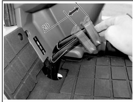
Push the clutch pedal down by hand, to measure the amount of pedal free movement.
