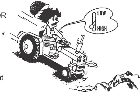
To start traveling, lower the engine speed and release the clutch pedal slowly.
