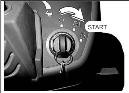
Turn key switch to start position until engine starts, but no more than 10 seconds, then release the key. Run engine for two minutes at 1500 RPM.
