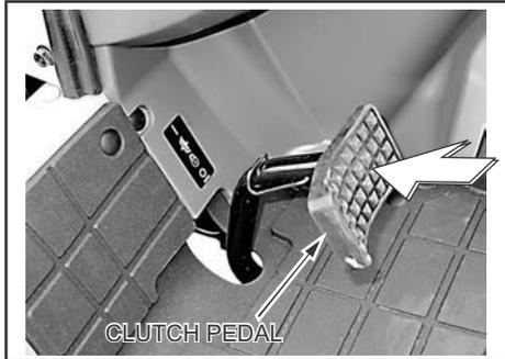
Push the clutch pedal down.
