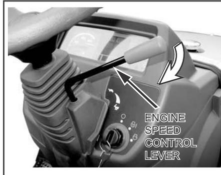
Put the engine speed control lever at the middle position.
