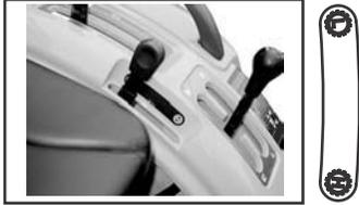
— Move the range shift lever forward to place the transmission in H range. Move the lever rear ward to place the transmission in L range.
