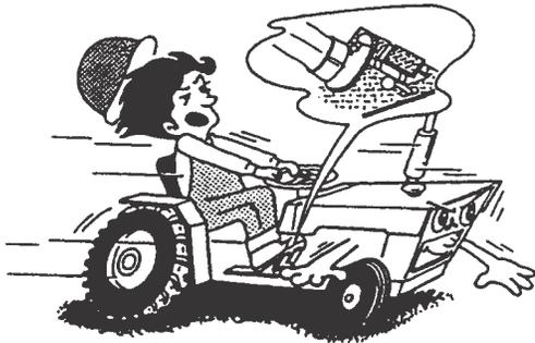
Never operate the differential lock while driving at high speed or traveling on the road. For driving the 4-WD tractor on the road, be sure to place the 4-WD shift lever in OFF position.
