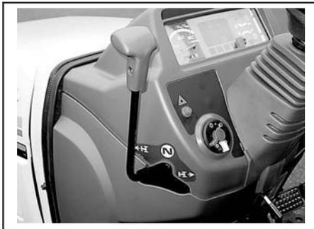
Put the SHUTTLE lever in the N (Engine start) slot (Gear Drive).
