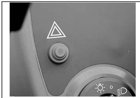
— To flash the Flasher Lamps whenever the tractor is operated or traveling onroads.
