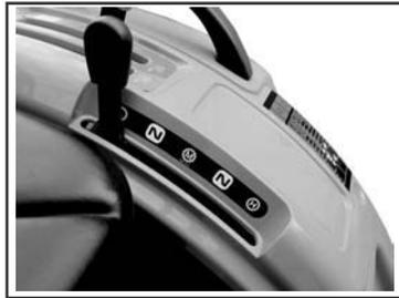
— Move the range shift lever forward to place the transmission in H range. Move the lever to the rearward to place the transmission in M or L range. The center position between M and L or H and M places the transmission in N.
