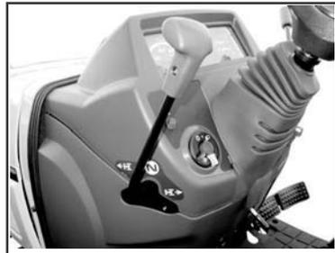
— The shuttle shift lever is used to shift the transmission gear into forward of reverse position. Move the shuttle shift lever forward (F position) to the forward position. Move the shuttle shift lever rearward (R position) to the reverse position. The center position between F and R places the transmission in N position. (neutral)
