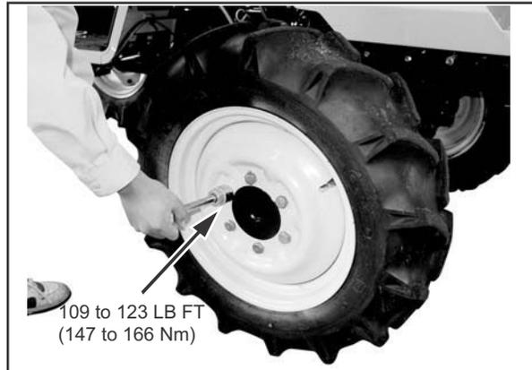
The front wheels are tightened with six bolts for MFD to the axle hubs.
