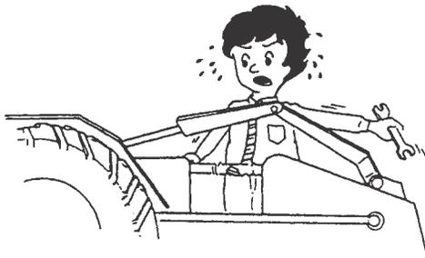
5. Never allows riders on the tractor, linkage drawbar or attachment while traveling and operating them.
