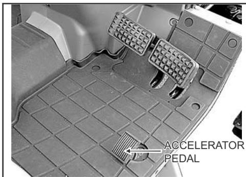
— Use this pedal when operating the tractor on the road. Push the pedal down to increase engine speed.
