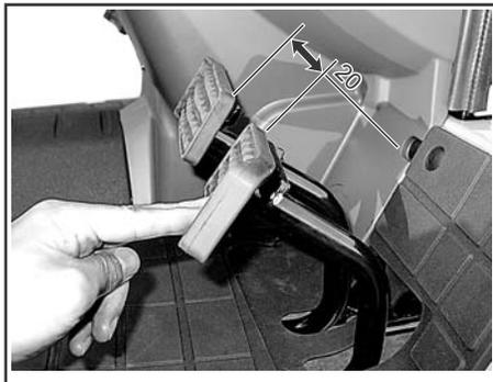
Loosen lock nut and rotate the brake rod to make a free play of 20 to 30 mm (0.79 to 1.18 in.) at the brake pedal. With this much play obtained, tighten the lock nut.
