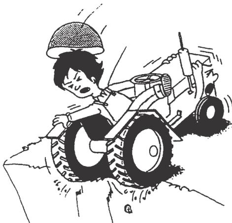
Avoid operating the tractor on an extreme slope that appears hazardous, when forced to operate on such slope, use extra care. Driving forward out of a ditch or mired condition or up a steep slope could cause tractor to tip over rearward.
