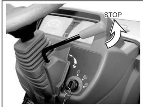
Move the engine speed control lever to run engine at idle speed for three to five minutes to decrease the temperature of engine.
