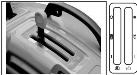
— Move the lever forward to engage the REAR PTO. Move the lever rearward to disengage the Rear PTO.
