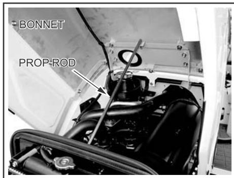
Lift the hood, and insert the Support Rod into hole.
