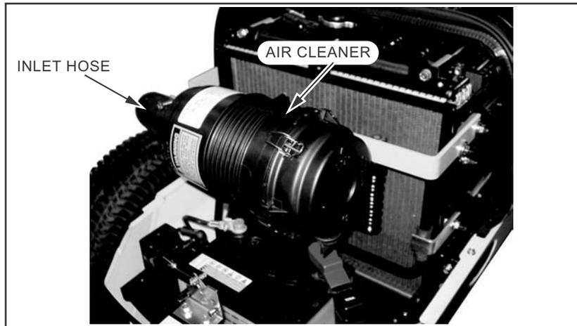
**IMPORTANT:** Service the air induction system at the given service intervals. Correct maintenance will add to the life of the engine. Keep all connections on the outlet hose tight.
