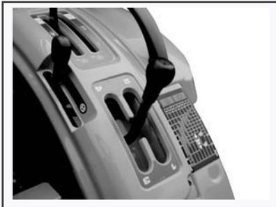
— The gear shift lever is used to shift the transmission gears into any of four speeds.
