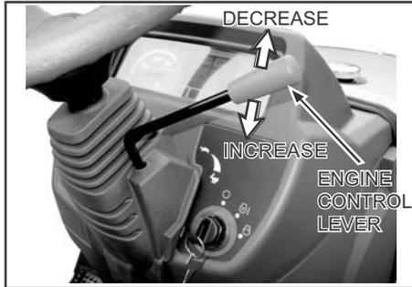
— Move the engine speed control lever to the rear to increase engine speed. Move the engine speed control lever forward to decrease engine speed.
