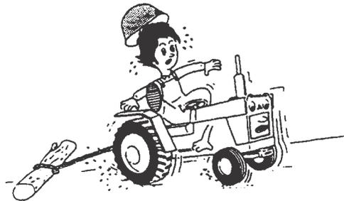
When operating the tractor on either a steep slope or flat ground, be sure not to suddenly steer, brake, clutch or operate attachments.
