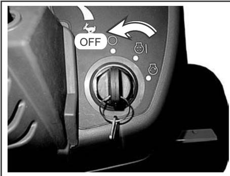
Turn the key switch to OFF position. Remove the key.
