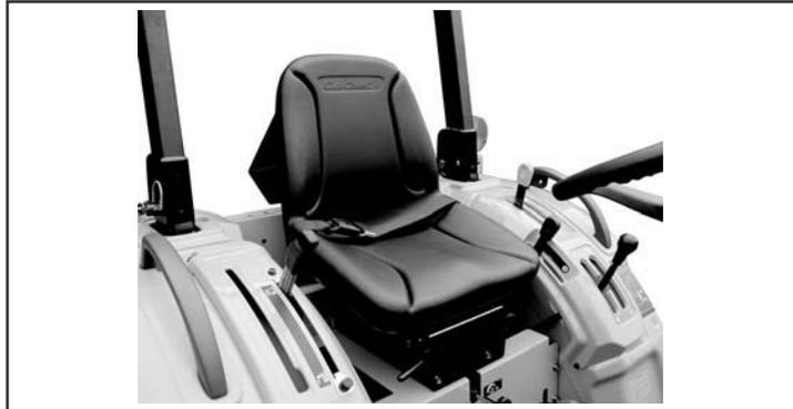
The seat is adjustable fore and aft by moving a lever.
