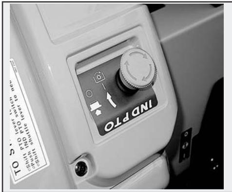
PTO switch is used to engage or disengage the Independent PTO clutch. Turn right to engage push to disengage.
