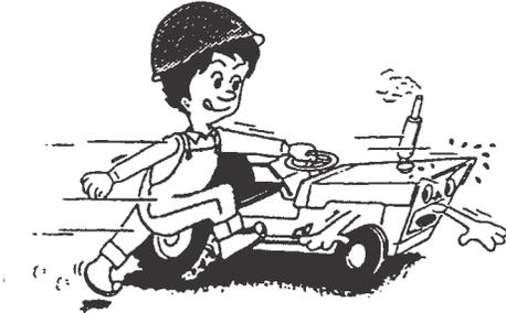
When starting the tractor, operating any attachment or engaging the PTO make sure that no one is in the way, especially children.
