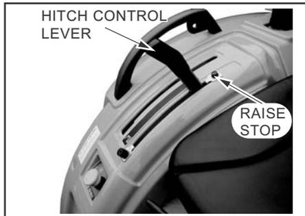
If raise stop setting position is incorrect, the hydraulic pump might be damaged. Therefore carefully adjust as below.
