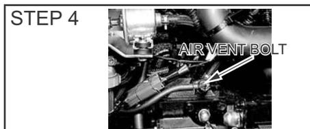
Loosen the air vent bolt on the injection pump and turn the key switch "ON" position until the fuel flowing from the pump is free of air bubbles. Tighten the air vent bolt.
