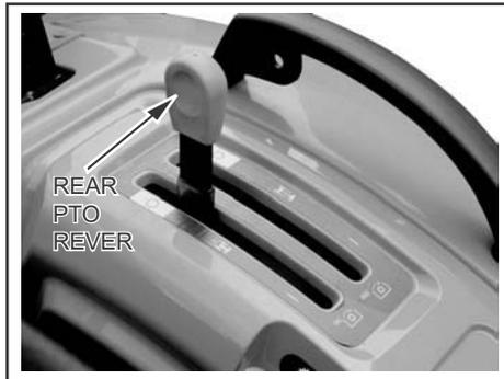
Put the REAR PTO control lever, MID PTO control lever and the range shift lever in the OFF or N (neutral) position.
