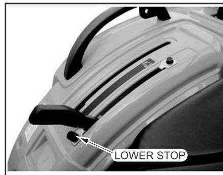
**IMPORTANT:** Position of the raise stop should not be set so rearward that insufficient free play of the lift arms is available at the highest position when hitch control lever is moved to the raise stop.
