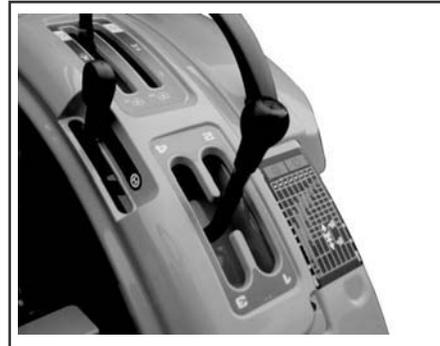
**NOTE:** When shifting from fourth to another range, be careful not to run the engine at more than 2700 RPM.
