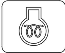
— This signal indicates the correct functioning of the glow plug circuit. When the glow plugs have reached the correct temperature for engine starting, the glow plug indicator lamp will be put out.
