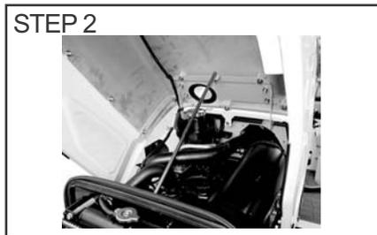
Lift the hood and connect the hood support rod.
