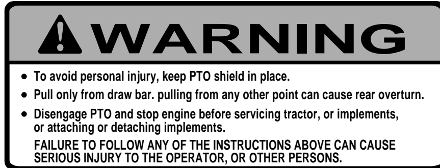
PTO WARNING LABEL LOCATED ON REAR PTO SHIELD
