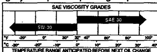
**NOTE:** Although multi-viscosity oils (5W30, 10W30 etc.) improve starting in cold weather, these multi-viscosity oils will result in increased oil consumption when used above 32°F. Check your engine oil level more frequently to avoid possible engine damage from running low on oil. Change after the first 25 hours of operation at least once a year if the lawn mower is not used for 25 hours in one year.
