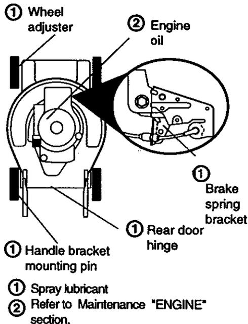
**IMPORTANT:** Do not oil or grease plastic wheel bearings. Viscous lubricants will attract dust and dirt that will shorten the life of the self lubricating bearings. If you feel they must be lubricated, use only a dry, powdered graphite type lubricant sparingly.
