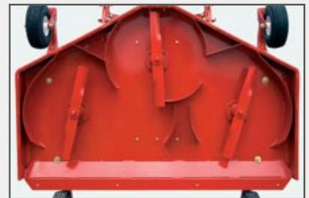
Each mower features three high-speed blades with one of the highest rated tip-speeds in the industry. This creates powerful suction that lifts the grass for a crisp cut. A blade overlap of 1 5/8" to 2 5/8" prevents stripping and ensures the lawn is mowed evenly.
