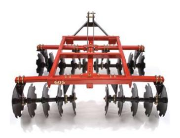
Disc: Frame - 2" x 3" x 1/4" wall tube Hitch - 1/2" x 3" flat iron. Discs spaced 7 ½" with cast iron spacers. Sealed, self-aligning bearings. 5 angle adjustments on each gang. All notched or smooth discs or combinations. Optional scraper kit and center sweep available.
