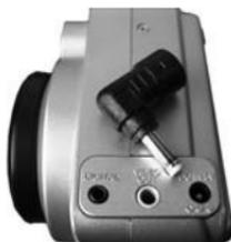
**WARNING:** myPower ALL Plus supports Center Positive polarity only. If your device has a Center Negative polarity, do not power the device with myPower ALL Plus; contact [support@tektron.com](mailto:support@tektron.com) for assistance.
