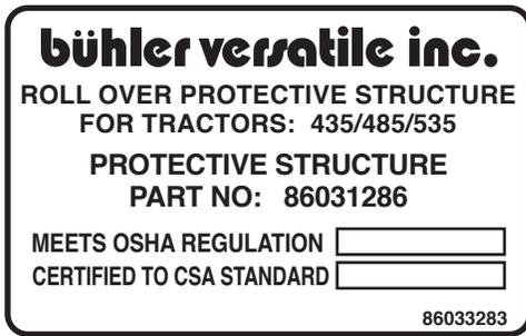
1. ROPS Certificate - Located left underside of cab.
