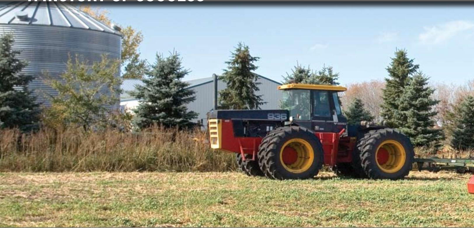
Versatile was the first company to mass-produce articulated four-wheel drive tractors, starting in 1966 with the D100 and G100 four-wheel drives. Those ground-breaking tractors were primitive by modern standards, with a 6-cylinder diesel or 8-cylinder gas engine producing 100 horsepower. 1966 models sold for less than CA\$10,000.
