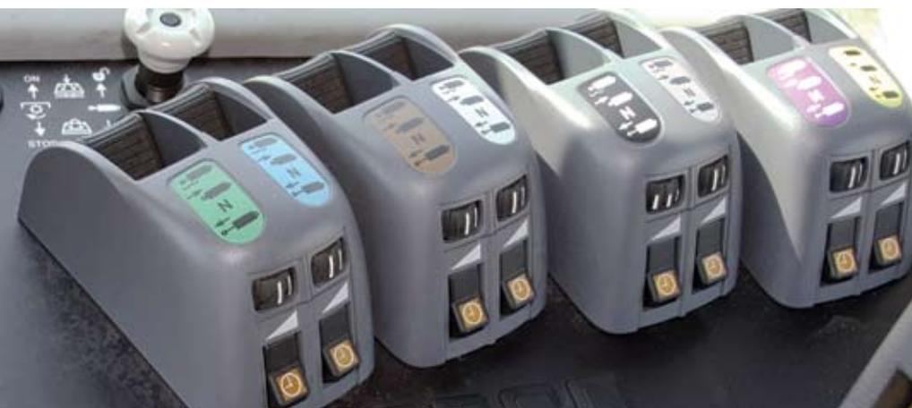
**Electro-hydraulics are available and feature fingertip controls to manage the raise, lower, float and neutral functions. Each remote has a convenient thumb wheel for precise flow settings and programmable timed self-centering detents.**
