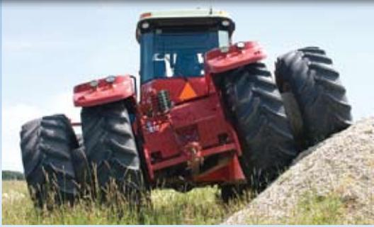
The planetary axles remain on the tractor during routine maintenance, limiting downtime. Daily inspections are easy with a quick visual check of the axle oil level indicators. The gears can also be reversed to extend the wear life.
