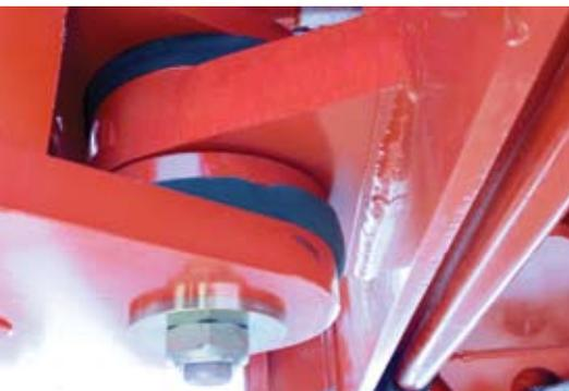
The drawbar pull point on Buhler Versatile four-wheel drives is immediately behind the articulation point, which now features a large-diameter pivot pin for maximum strength and durability. Models 305, 340, 375 and 400 feature a 2.36" (60 mm) pivot pin while the High Horsepower Tractor Series have a 3.15" (80 mm) pivot pin.
