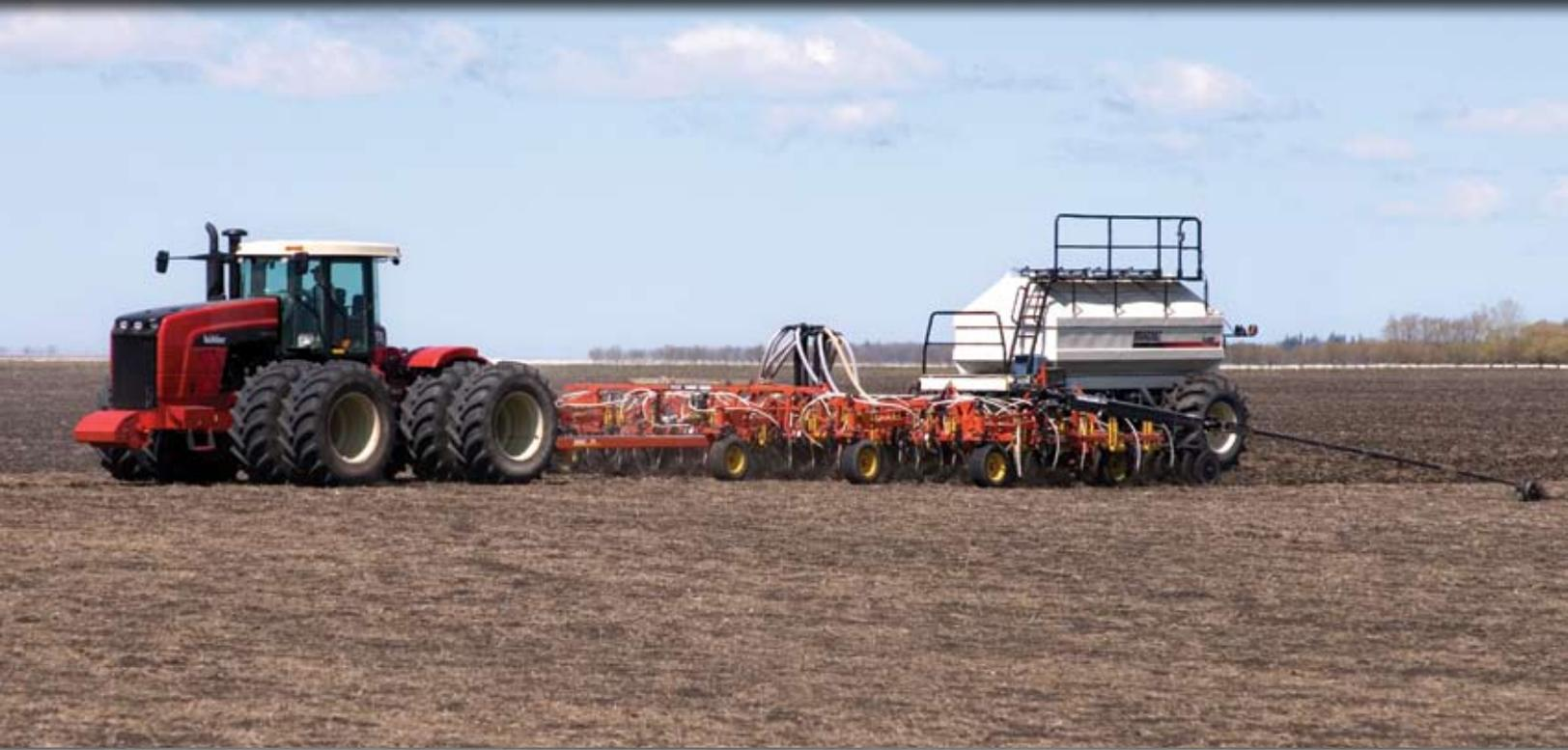
Modern implements require more hydraulic capacity to operate efficiently and the hydraulic system on Buhler four-wheel drive tractors has been developed to meet those demands. The closed center load sensing hydraulic system provides ample capacity for implements that demand high hydraulic flow by providing pressure and flow on demand. When no hydraulic power
