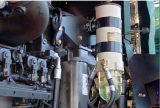
**A large auxiliary fuel filter is standard equipment. With a larger capacity, the fuel filter ensures that fuel is thoroughly filtered to ensure harmful debris is removed before entering the engine, which is particularly important when using biofuels. This filter is visible from the ground or from the entry platform for easy inspection.**
