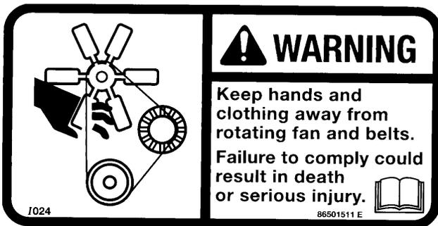
13. Engine Cooling Fan - Located under the engine side shields.
