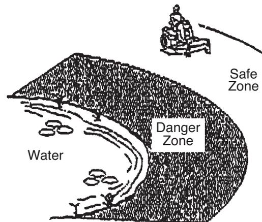
1. Use EXTREME caution when mowing and/or turning on slopes as loss of traction and/or tip-over could occur. The operator is responsible for safe operation.
