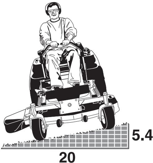
Operation on slopes can be dangerous. Using the unit on a slope that is too steep where you do not have adequate wheel traction (and control) can cause sliding, loss of steering, control, and possible rollover. You should not operate on a slope greater than a 5.4 foot rise over a 20 foot length (15 degrees).
