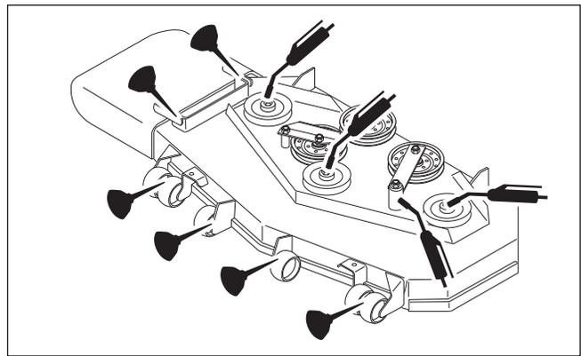
Figure 20. Deck Lubrication
