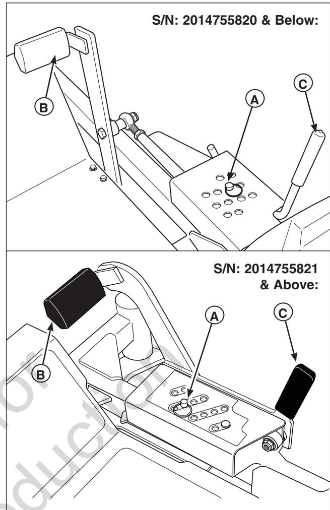
Figure 6. Mowing Height Adjustment
