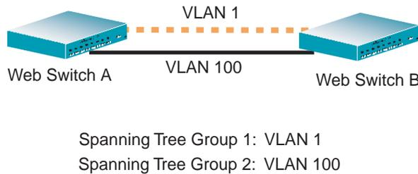
**Figure 2-3** Using Multiple Instances of Spanning Tree Protocol
