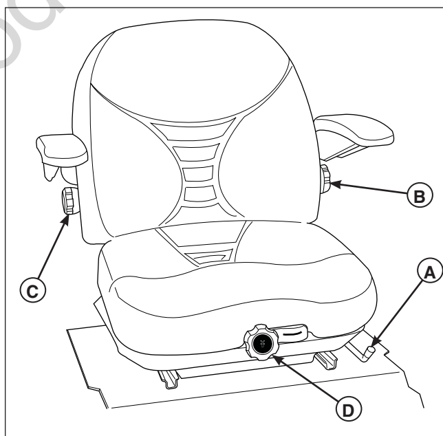
Figure 5. Suspension Seat Adjustment A. Forward / Backward Seat Adjustment Lever B. Lumbar Adjustment Knob C. Back Angle Adjustment Knob D. Suspension Adjustment Knob
