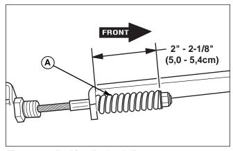
Figure 31. Parking Brake Adjustment A. Upper Brake Spring
