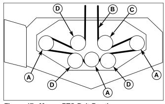
Figure 47. Mower PTO Belt Routing
