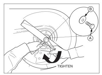
Figure 24. Installing The Blade
