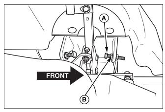
Figure 28. Top Speed Adjustment A. Top Speed Adjustment Bolt B. Flange Nut
