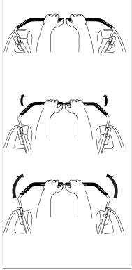
Figure 3. Move Control Levers Gradually
