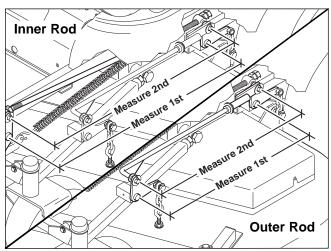
Figure 38. Measure the Inner & Outer Lift Rods
