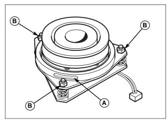
Figure 34. PTO Clutch Adjustment A. Adjustment Window (Qty. 3, one shown) B. Adjustment Nut
