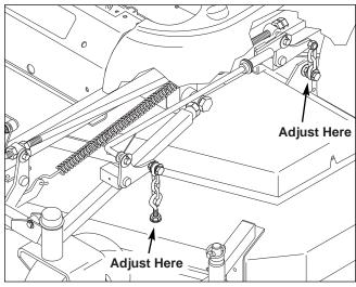
Figure 42. Deck Level & Spring Length Adjustment
