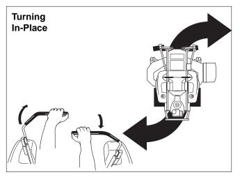
Figure 7. Turning in Place
