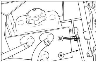
Figure 29. Neutral Adjustment A. Adjustment Linkage Rod B. Nuts
