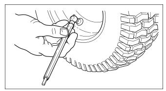
Figure 11. Checking Tire Pressure
