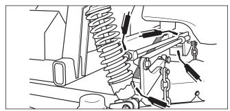
Figure 16. Deck Lift Linkage Pivots
