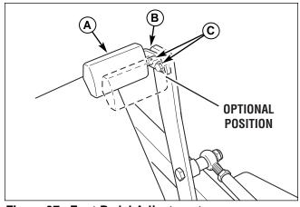
Figure 37. Foot Pedal Adjustment
