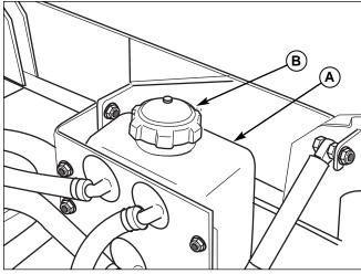
Figure 13. Checking Hydraulic Oil Level
