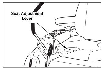
Figure 25. Seat Adjustment
