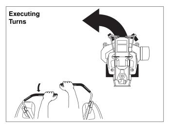
Figure 6. Turning Around a Corner
