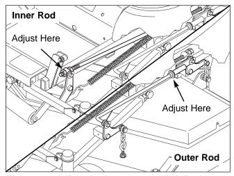
Figure 40. Adjust the Inner & Outer Lift Rods
