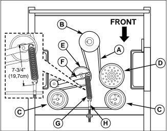
Figure 44. Hydraulic Pump Drive Belt Replacement
