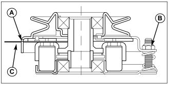
Figure 35. Adjust PTO Clutch
