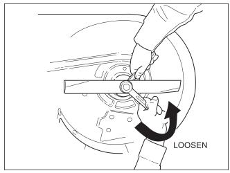
Figure 22. Removing the Blade
