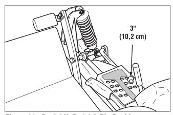
Figure 39. Deck Lift Pedal & Pin Position
