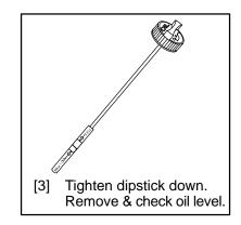
**Oil filling procedure:** first add 1 quart (32 ounces or 1 liter). Start and run engine at idle for 30 seconds. Shut engine off and wait 30 seconds. Then add more oil slowly to bring level to **Full** mark on dipstick.
