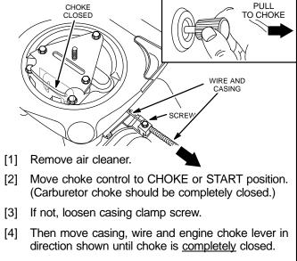
[5] Tighten casing clamp screw. Replace air cleaner.
