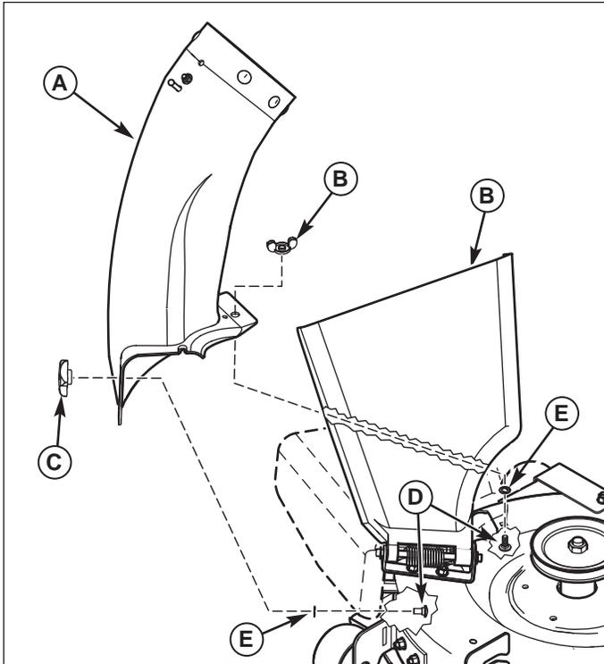
**Figure 7. Install Chute**
