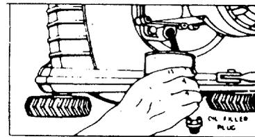
Change oil after first 5 hours of operation while engine is warm. Thereafter, change oil every 25 hours of operation while engine is warm. Engine may be drained through oil filler opening. Be sure to replace drain plug and oil filler cap.
