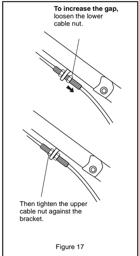
To decrease the gap between the friction disc and the aluminum drive plate:
