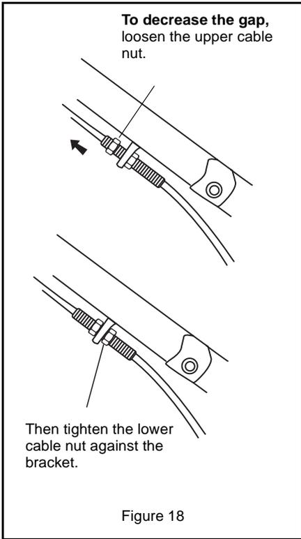
2. Check the adjustment and readjust as needed.
