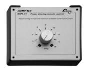
For instance if the source is a generator of 2000 Watt, the potentiometer has to be set at max. 8A. This value is obtained in dividing 2000 Watt by 230V. If the HP-COMPACT is connected to a power source which is protected by a 6A circuit breaker, the potentiometer must be set at a max. value of 6A.
