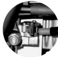
Fuel shutoff valve closed.
