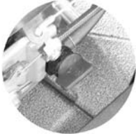
Fuel shutoff valve open.
