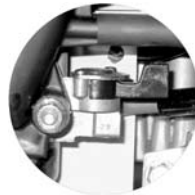
Fuel shutoff valve open.
