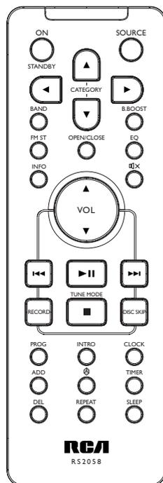
**ON/STANDBY** - Turns power on or off (STANDBY mode).
