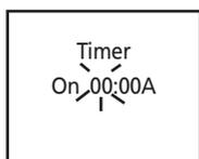
2. For setting time, press **◀▶** or **▶▶** to set the hour and then press **TIMER** to shift to minute digits.
