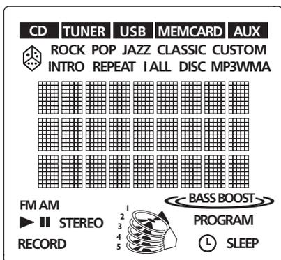
**CD / TUNER / USB / MEMCARD / AUX** - indicates the current mode.
