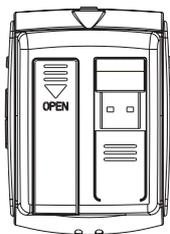
2. Insert a "AAA"(UM4) battery with polarities corresponding to the indications in the compartment. (Refer to "Before You Begin" for important battery information.)
