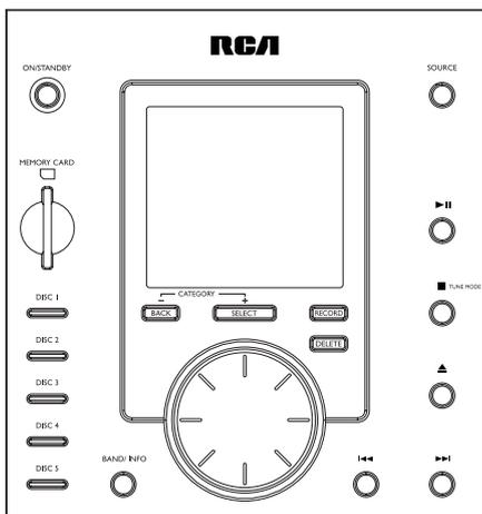
**ON/STANDBY** - Turns power on or off (STANDBY mode).
