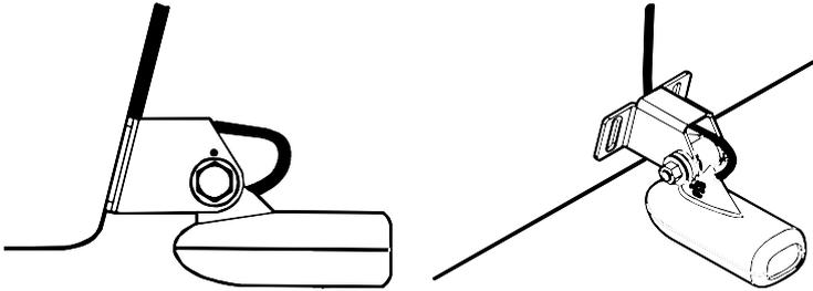
**Route cable over bolt and through bracket. Side view shown at left and seen from above at right.**
