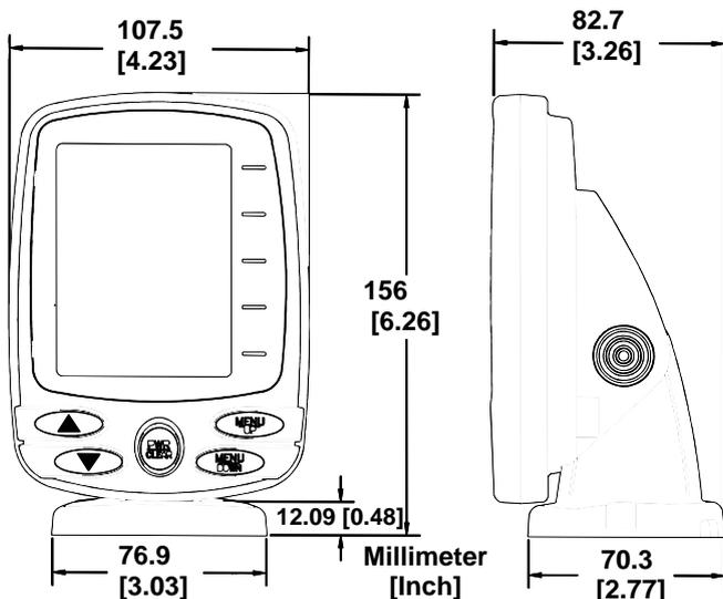
**Front view (left) and side view (right) showing dimensions of the X37TX and X47TX when mounted on quick release bracket. The swivel base (not shown) adds 0.4" (10 mm) to the height. The swivel base width is 4.25" (10.7 cm) and the depth is 3.12" (79.47 mm).**
