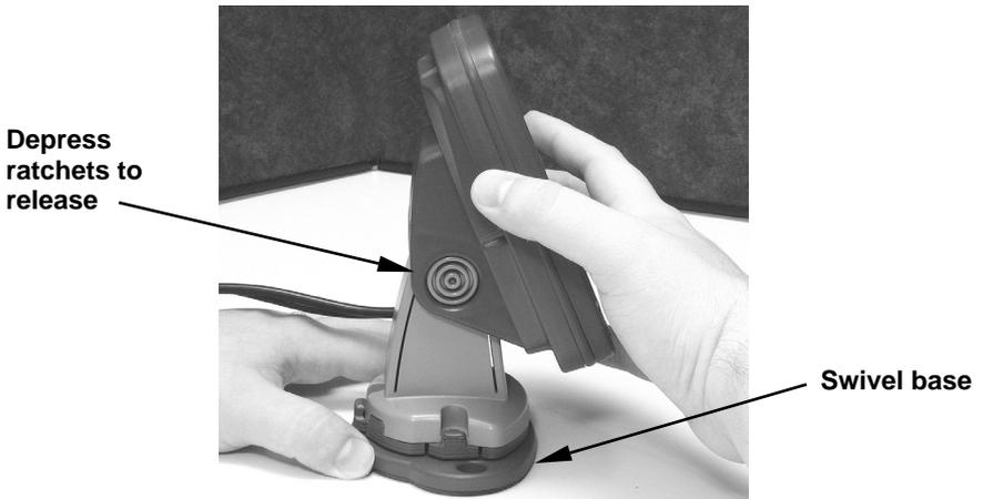
**Adjust viewing angle: use one hand to press and release the spring-loaded ratchets while you move the unit with the other hand.**
