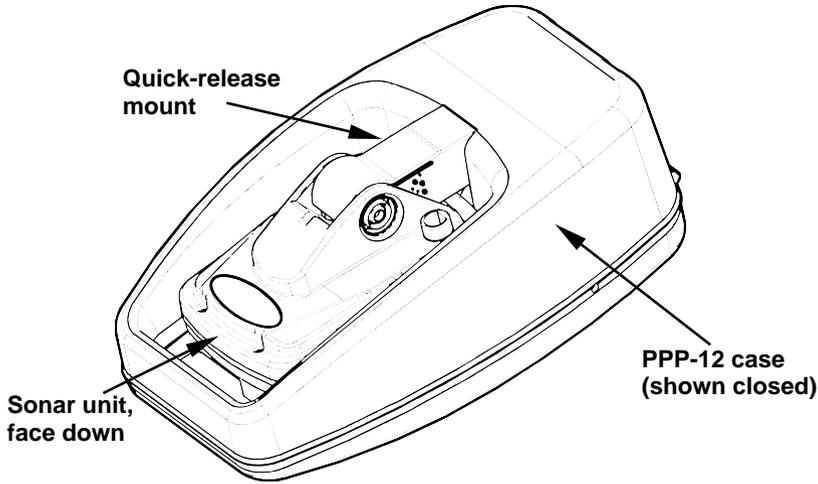
**Place the unit on the quick-release mount. The unit can be folded down into the "Closed" position (as shown) for convenience in storing or transportation, as well as for the protection of the unit.**
