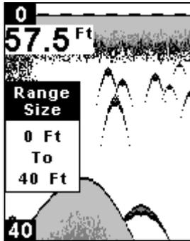
**Range Size** menu with manual depth range set to 40 feet. This in effect "zooms" or enlarges the display to show the water column from 0 to 40 feet deep. In this figure, the boat is in 57.5 feet of water, but only the top 40 feet of the water column is shown on the screen.
