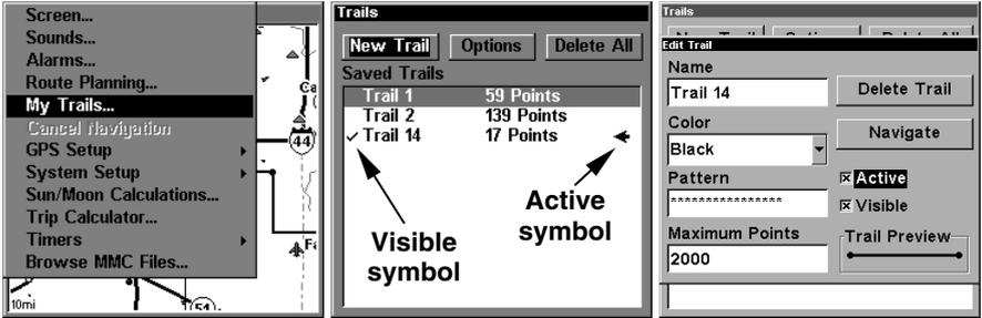
Sequence for saving a trail and beginning a new one. At left, My Trails command. Center, the Trails Menu. The arrow to the right of Trail 14 indicates the trail is "active," and the check to the left indicates the trail is visible on the map display. The right figure shows the Edit Trail menu, with the Active command selected.
