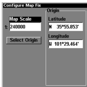
**Configure a map fix so LMS-320 can find your position on a printed chart or topographical map.**
