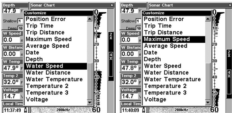
Options List for customizing Digital Data windows. At left, the list first appears with Water Speed selected. At right, Maximum Speed has been picked to replace Water Speed in the top digital data window.
