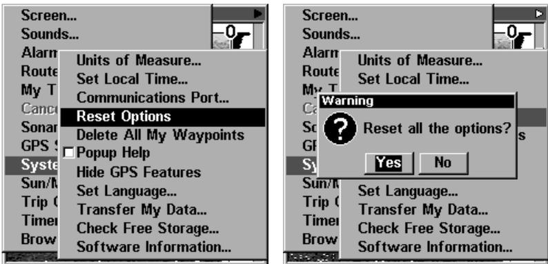
At left, System Setup menu with Reset Options command selected. At right, the Reset Options dialog box, with "Yes" selected.
