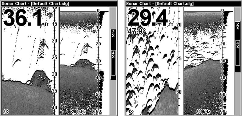
Split Zoom Sonar Chart. Image at left shows the left window zoomed to 2X. The right image shows the left window zoomed to 4X. The depth overlay data is set to the default large text size; the water temperature is set to the small text size.
