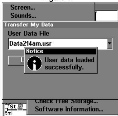
These figures show the menu sequence for loading a GPS Data File from an MMC into LMS-320's memory.
