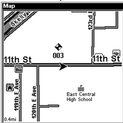
Sequence for setting a waypoint. Step 1: while traveling, *quickly* press **WPT twice** to call up Find Waypoint screen (seen in Step 2) and set a point. Step 3: a message says the waypoint has been saved. Step 4: vehicle continues on its way; number waypoint symbol is visible on map.
