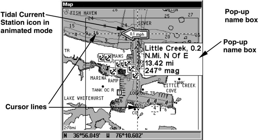
Navionics chart showing Tidal Current Station icon selected by cursor. In this example, the tidal current is in flood but it's about to enter the slack water stage. The current is flowing to the west at 0.1 mph.
