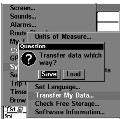
The Transfer My Data submenu asks if you want to save data to the MMC or load data from the MMC into LMS-320's memory.
