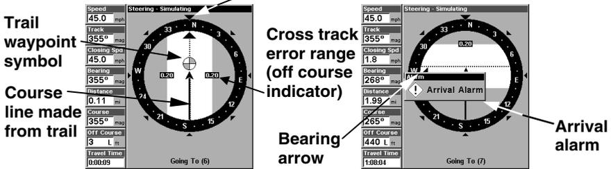
Navigate trail, navigation page (compass rose) views: at left, driver is northbound heading straight toward trail point 6; bearing arrow shows the trail point is due north (straight ahead.) At right, driver has reached trail point 6 and must turn west to follow the trail. Arrival alarm goes off and bearing arrow swings around to say turn left (west), toward the next waypoint, trail point 7. LMS-320 now shows navigation information to point 7, which is 1.99 miles away.
