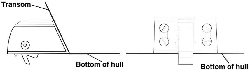
**Speed sensor mounting configuration:
