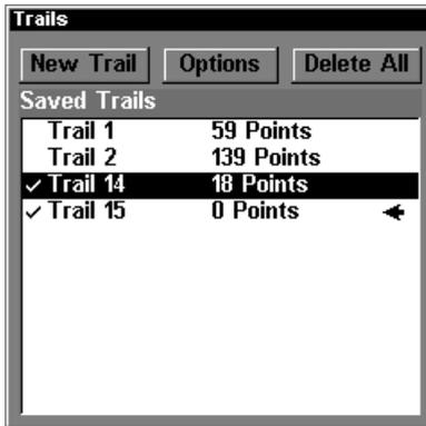
New trail, named "Trail 15," is created when Trail 14 is made inactive. Any new travel will be recorded in this trail, which is active and visible. Trails do not need to be visible in order to be active.
