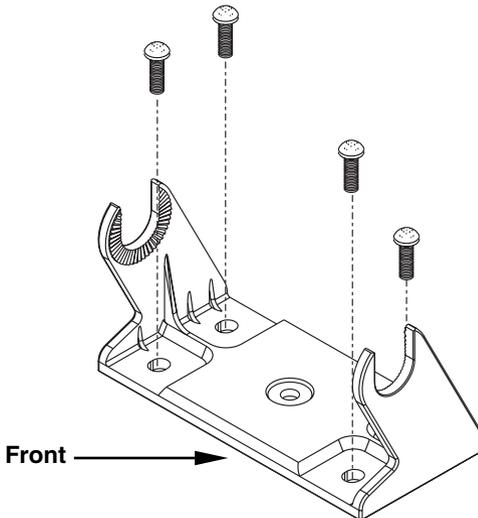
**Install the gimbal bracket. Orient the bracket so the arms slope toward the front of your unit.**
