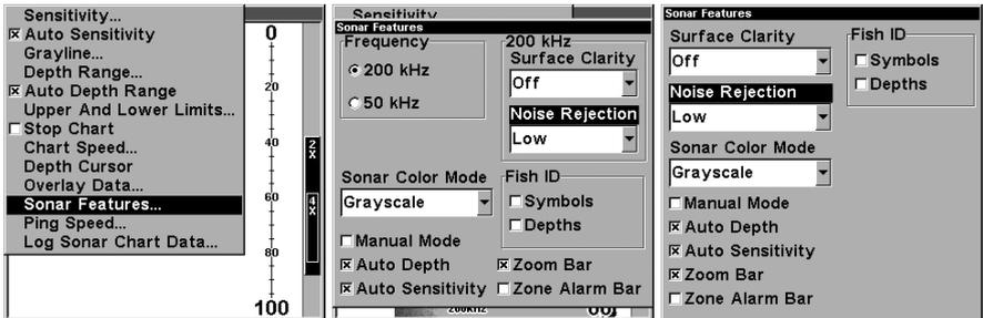
At left, Sonar Menu with Sonar Features selected. In the Sonar Features menu, Noise Rejection is selected with ASP in the default low setting (center, dual-frequency menu; at right, single-frequency menu).
