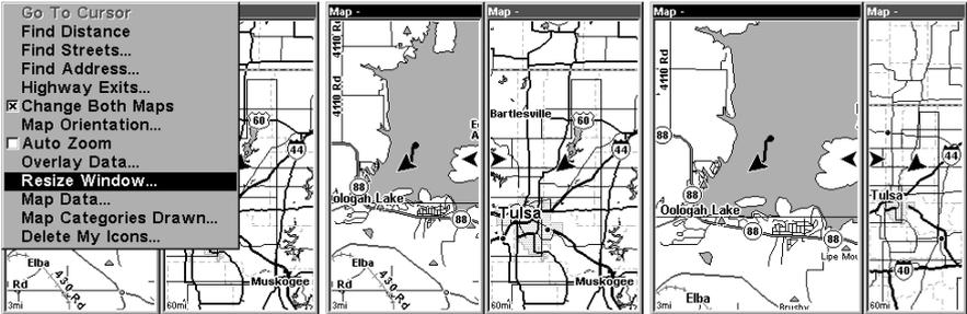
At left, Map Menu with Resize Window command selected. Center, Resize Window command is active. At right, pressing the → key moves the centerline to the right and enlarges the left window.
