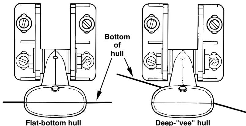
Align transducer centerline with hull bottom and attach transducer to transom. Rear view of dual-frequency Skimmer shown.
