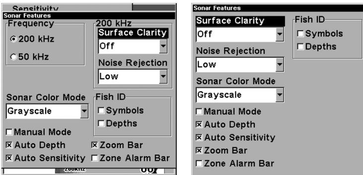
Sonar Features menu with Surface Clarity selected (at left, dual-frequency menu; at right, single-frequency menu).
