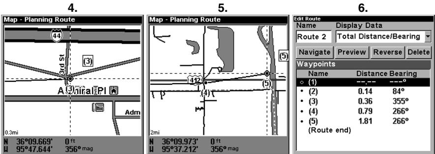
Route creation sequence, continued: Fig. 4. Point (3) set at on-ramp turn. Fig. 5. Waypoint (4) set at highway exit to frontage road leading to river. Waypoint (5) ends the route at a tree stand in the hunting area. Fig. 6. Press **EXIT** to save the route and you return to this screen.
