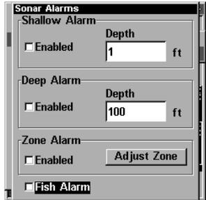
Sonar Alarms menu with Fish Alarm selected. The check box to the left is blank, indicating the alarm is turned off.
