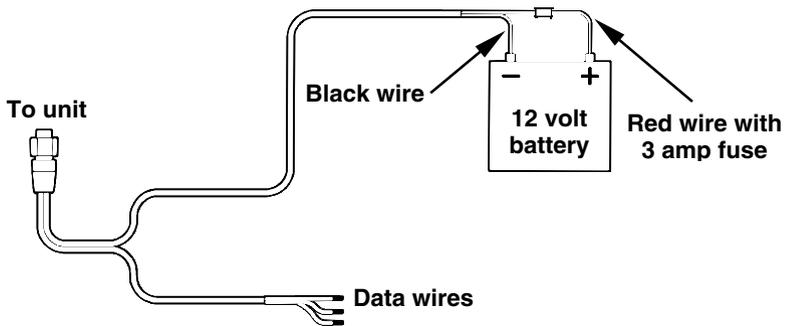
**Power connections for the LMS-320 series sonar/GPS unit.**
