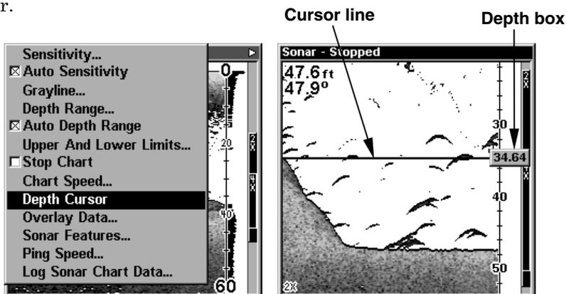
At left, Sonar Page menu with **Depth Cursor** command selected. At right, sonar chart with the depth cursor active. The line indicates the large fish is 34.64 feet deep.
