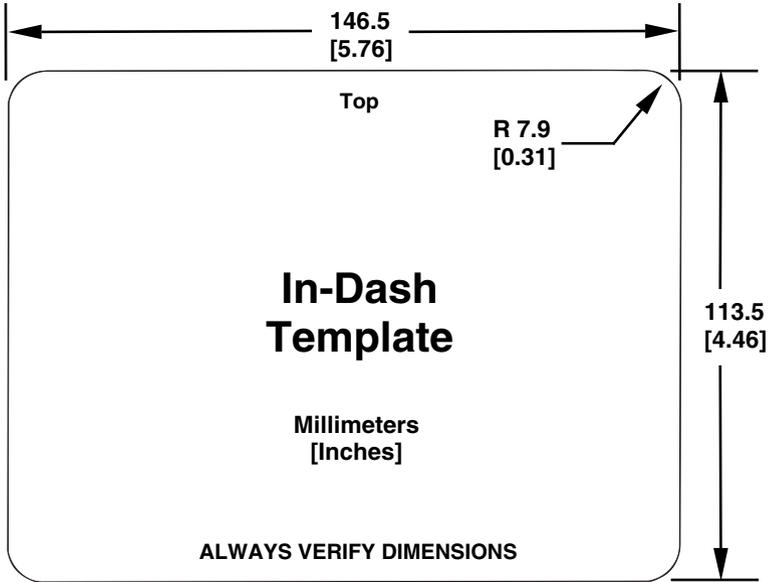
**In-dash mounting template for LMS-320 sonar/GPS unit, showing dimensions. NOTE: The figure above is *not* printed to scale. A scaled template (FM-5 In-Dash Adapter Kit instructions) is available for free download from our web site, [www.lowrance.com](http://www.lowrance.com).**
