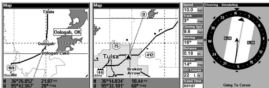
The 15-mile zoom figure at left clearly shows the dotted course line connecting your current position to your destination. The 40-mile zoom, center, shows both current position and destination on screen.
