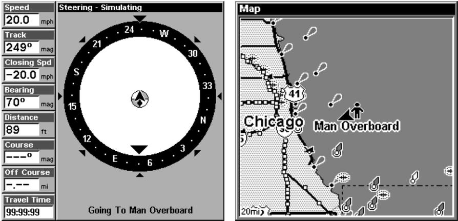
Navigating to Man Overboard: Navigation Page, left, and Map Page, right. The victim is astern of the vessel; the GPS shows which direction to steer to for the rescue.
