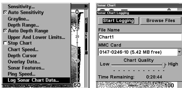
At left, the Sonar Page menu with the Log Sonar Chart Data command selected. At right, Sonar Chart Logging menu, with the Start Logging command selected. The menu says the MMC has 5.42 MB of free space, which will record the scrolling chart for 28 minutes and 44 seconds.
