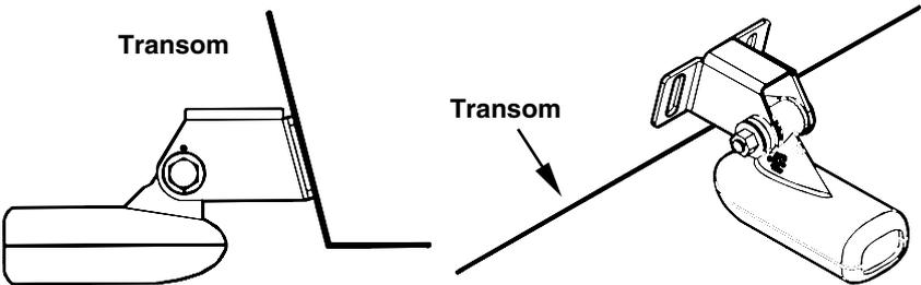
Position transducer mount on transom and mark mounting holes.
