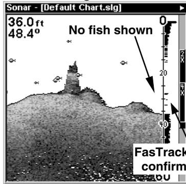
At left, figures 1A and 2A show Sonar Page in normal chart mode. At right, figures 1B and 2B show the same underwater scene with Fish I.D. turned on. Note how arches are replaced with symbols.
