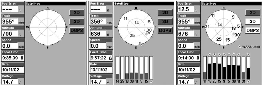
**Satellite Status Page. Left view indicates unit has not locked on to any satellites and does not have a fix on its position. Center view shows satellites being scanned. Right view shows satellite lock-on with a 3D position acquired (latitude, longitude and altitude), and WAAS reception.**
