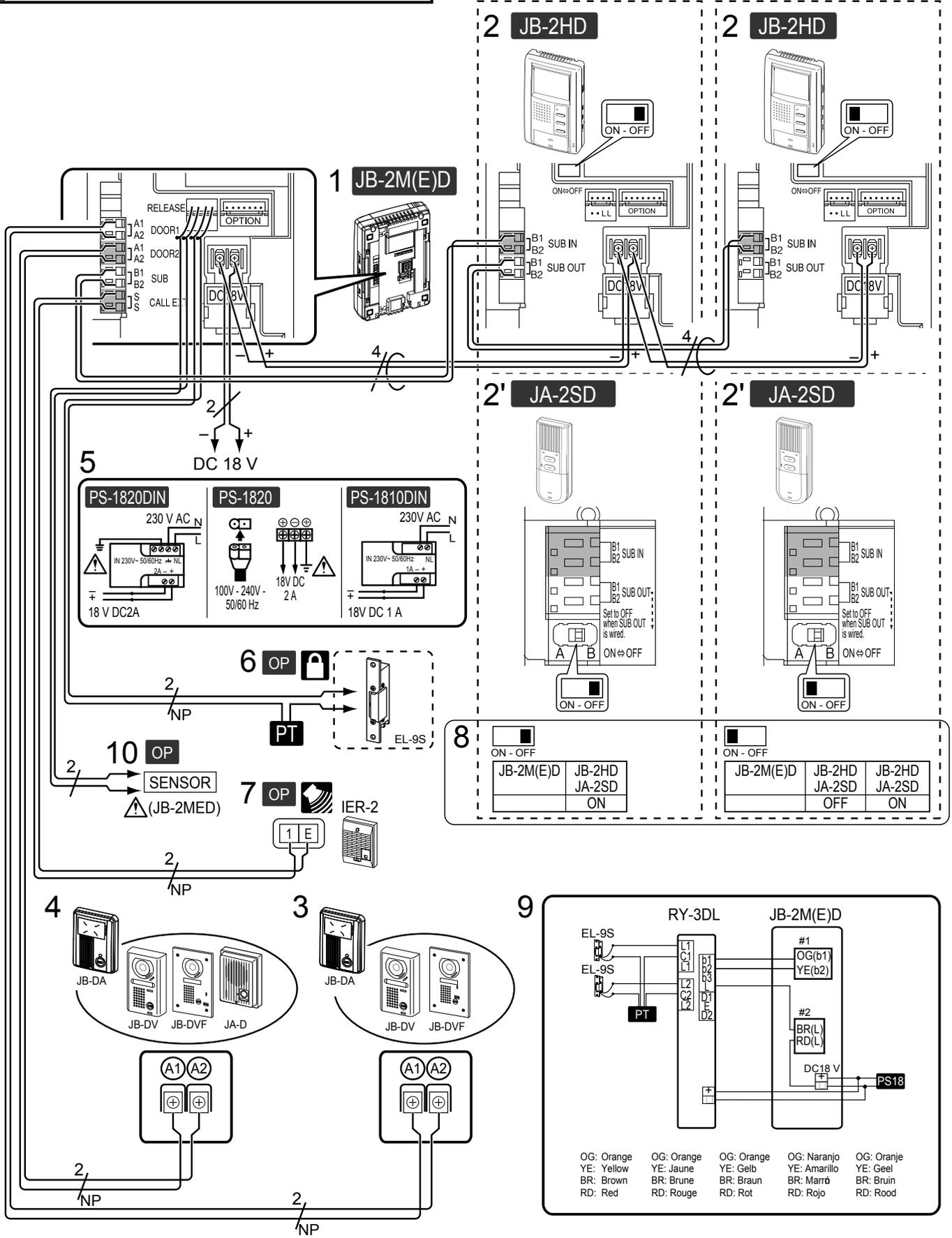
Securely insert wires into each terminal as shown.
