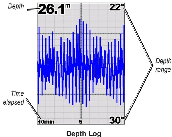
The depth appears along the right side, and the time elapsed appears along the bottom. The graph scrolls to the left as information is received.
