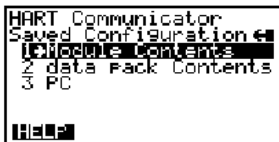
FIGURE 1-18. Saved Configuration Menu (Offline).
