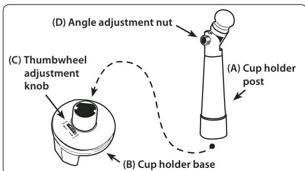
Step 2. Place the Cup Holder Mount into the designated cup holder in the vehicle. Adjust the thumbwheel adjuster (C) to open or close the cup holder prongs to fit in the cup holder.
