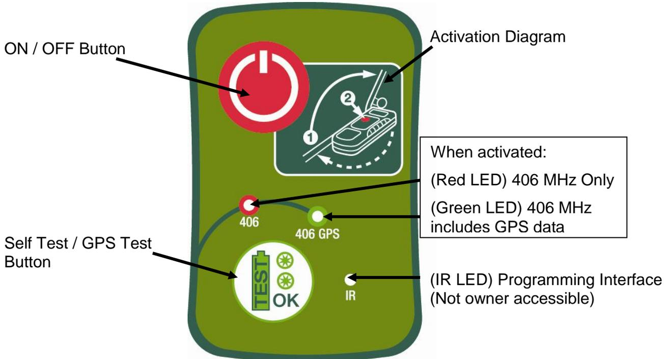
**NOTE:** If you notice the PLB is flashing the red or green LED and BEEPING periodically on its own, this likely means it has accidentally been activated and needs to be shut off and reported.
